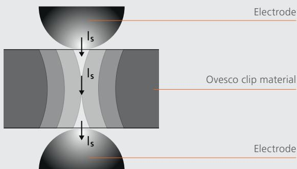
The remOVE DC Impulse generates a bipolar direct current pulse. This direct current pulse is applied to the Ovesco Clip using the remOVE DC Cutter. This causes local melting and severing of the clip, which is best done at the thinnest part of the arches.
