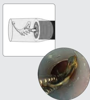
Use the remOVE Grasper to pull the clip fragments into the remOVE SecureCap and remove them from the digestive tract.
