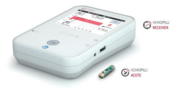
The HemoPill® acute is quick and easy to use: The capsule is connected to the receiver and swallowed by the patient. The capsule then moves along the GI tract through peristalsis. The maximum measurement time is 9 hours.
