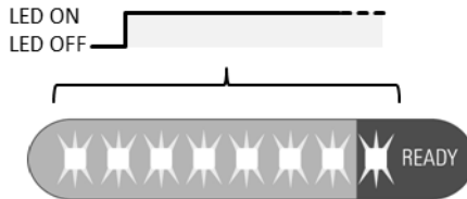
Figure 8: Status display indicates operational readiness through emitting constant green light from all eight LEDs.
